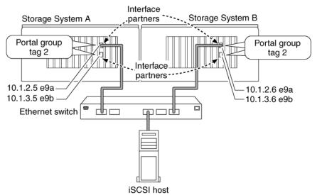
Storage System B has the same Ethernet card in slot 9. Interface e9a is assigned 10.1.2.6, and e9b is assigned 10.1.3.6. Again, the two interfaces are in a user-defined target portal group with tag value 2.
